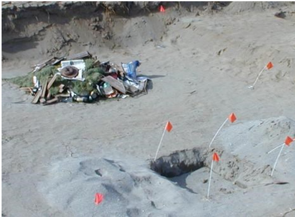
Fig. 9. Trash pile and un-burned earth oven (in the foreground) in the medium depth of the test bed. The trash pile contains many metal objects that reflect radar energy, but the earth oven was un-fired and therefore did not have a surface from which to reflect energy.
