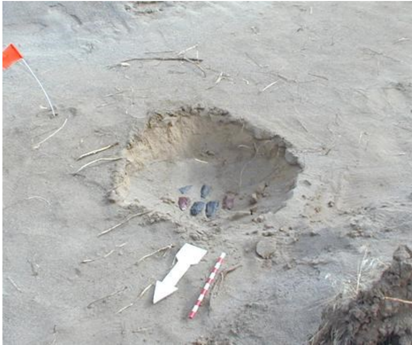
Fig. 10. Cache of lithic materials in the shallow depth of the test bed. These small artifacts reflected no radar energy as they are too small.
