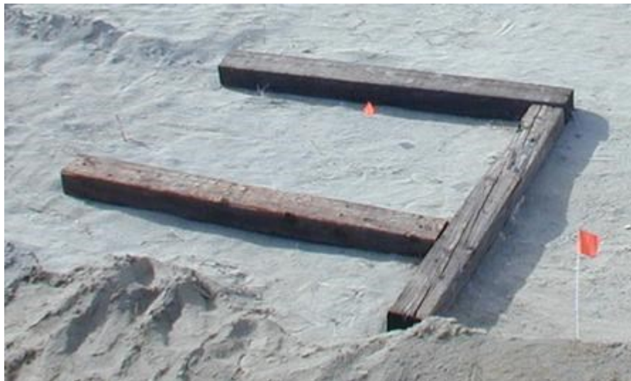
Fig. 12. Railroad ties in the deepest portion of the test bed that produced no reflections when the ground was dry. When the ground had been saturated with water and then left to drain for 2 days, these ties retained water (like a porous sponge) while the water drained readily from the surrounding sand. The wet railroad ties reflected radar waves when they were saturated.
