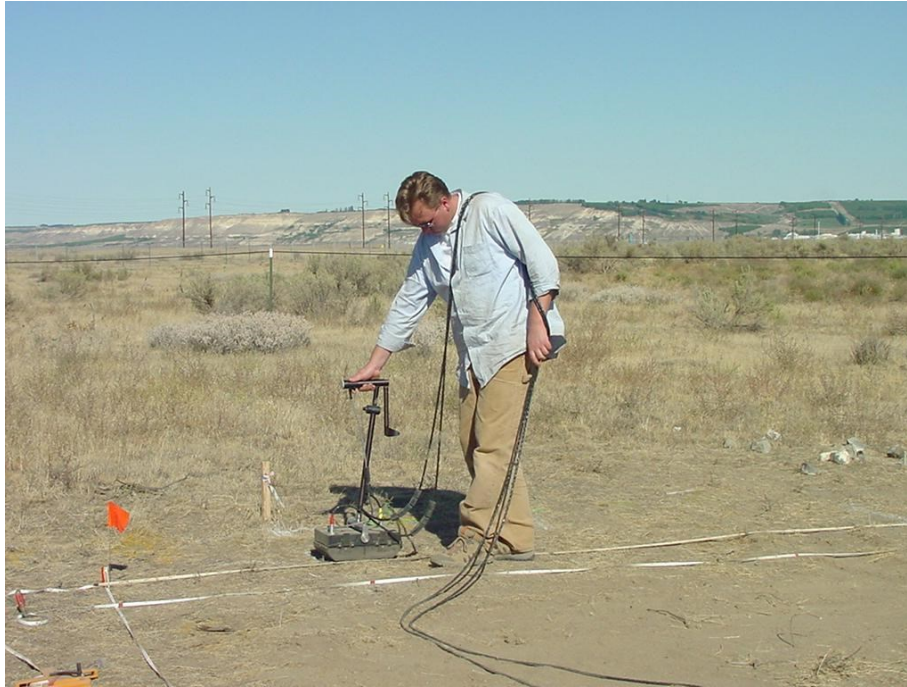
Fig. 4. Collecting GPR reflection data with a Sensors and Software 500 MHz antenna.
