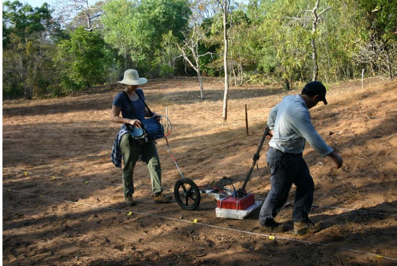
Figure 4: Collecting 400 MHz GPR reflection profiles.
