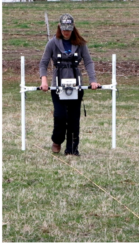
Figure 6: A Bartington 601-2 Fluxgate gradiometer used for magnetic data collection.
