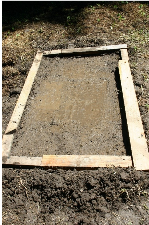
Figure 3: Creation of the footprint model in Oregon, with the boards outlining the test grid that was 180 x 100 cm in dimension.
