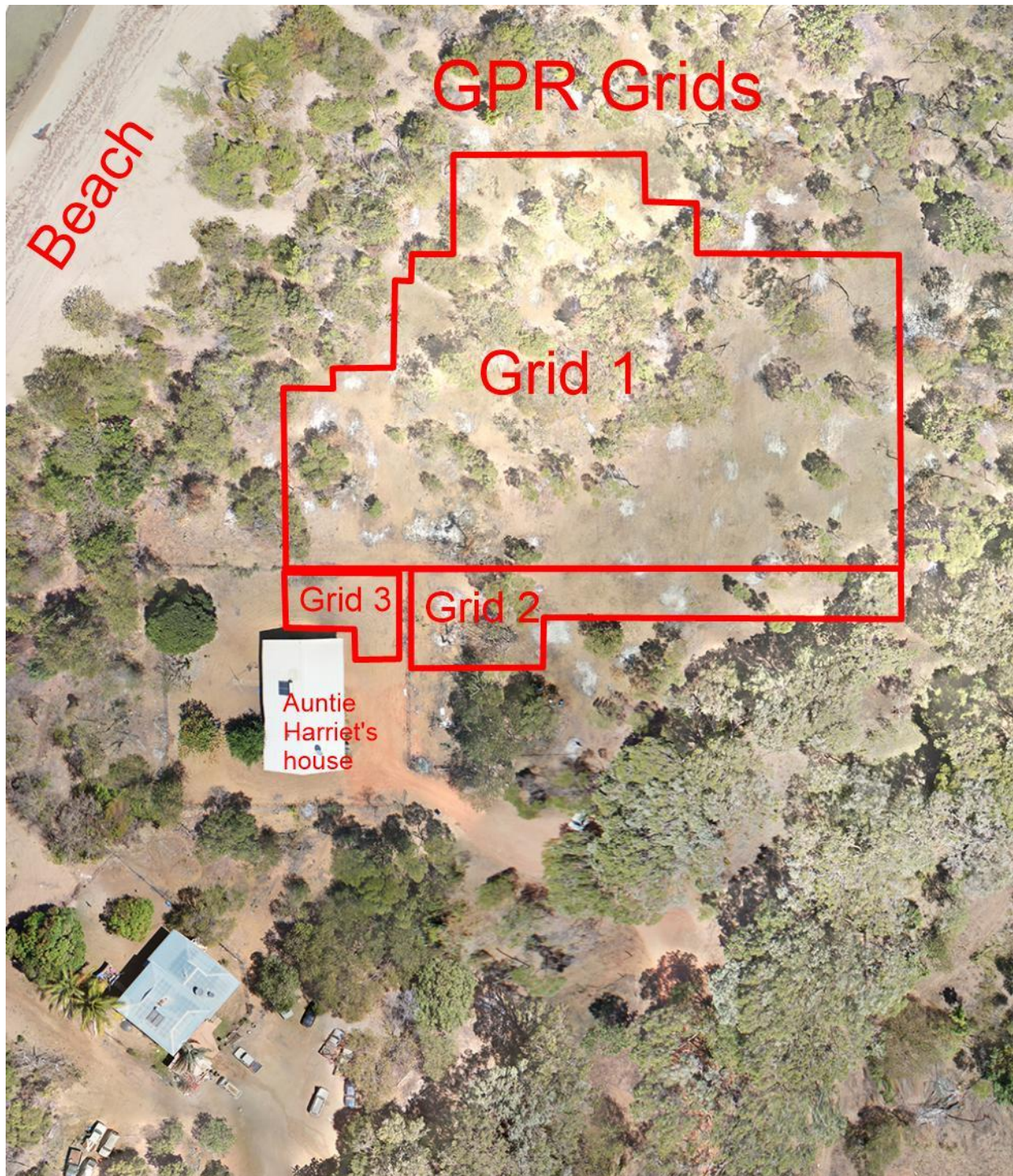
Figure 13: Location of GPR grids at the Mapoon Mission Cemetery. The 0,0 datum for the site grid is in the southwest corner of Grid 1. Every grave is measured from that point.
