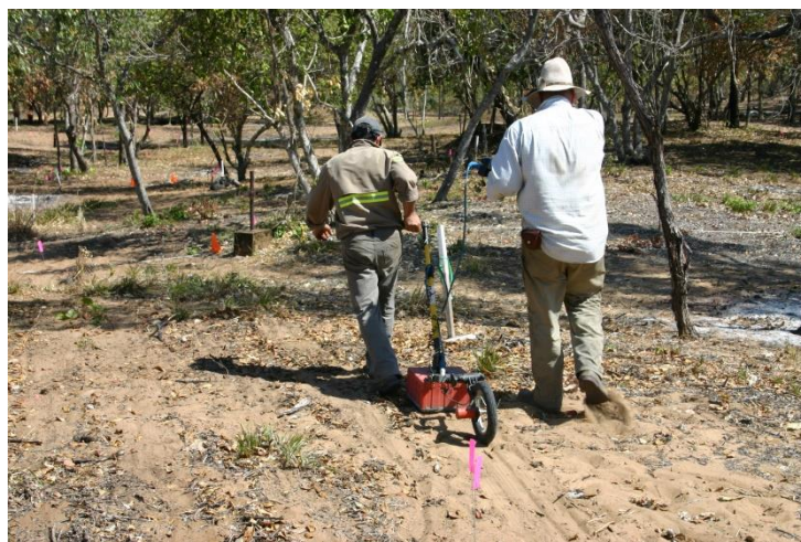
Figure 6: Collecting GPR data with the SIR-3000 system and 400 MHz antennas with survey wheel attached for distance measurement.
