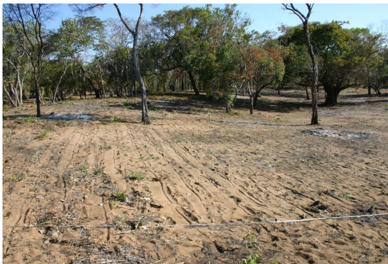
Figure 7: Marks on the sand from GPR antenna transects 50 centimeters apart.
