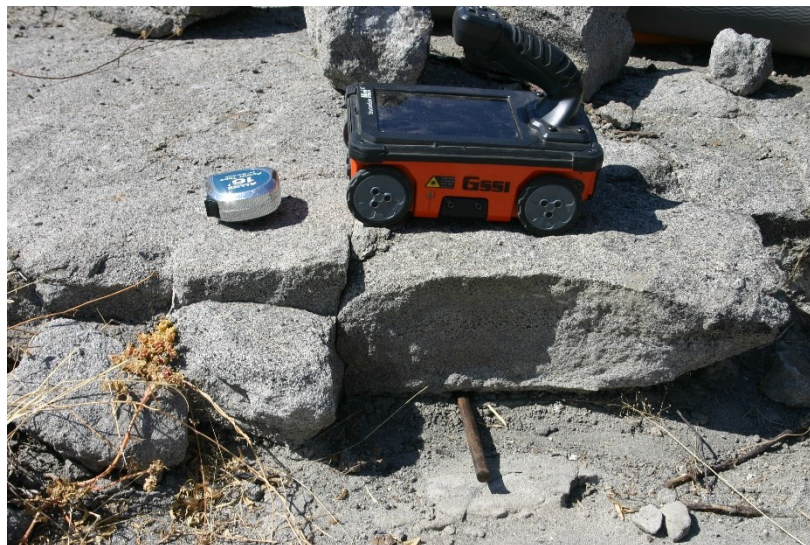
Figure 1: Conducting a velocity test with an iron bar placed at the T-7-T-8 contact.
