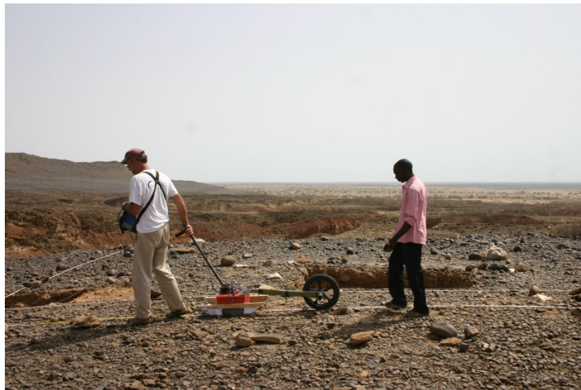
Figure 2: Collection of GPR profiles at Lothogam North using the 400 MHz antenna and a survey wheel for distance calibration. The trench for velocity and stratigraphic calibration is just beyond the antenna.
