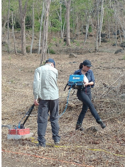
Figure 3: Collecting 400 MHz profiles in leaf-litter that covers the ground in this dry tropical forest in April.
