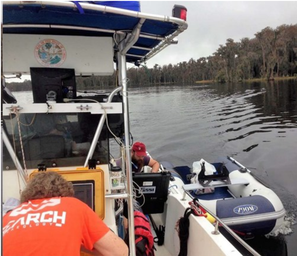
Figure 3: Collecting data at Newnan's Lake. The GPR unit is in the stern an inflatable boat (far right). It is important that these craft not have inflatable bottoms, as the air pockets will disrupt radar waves.
