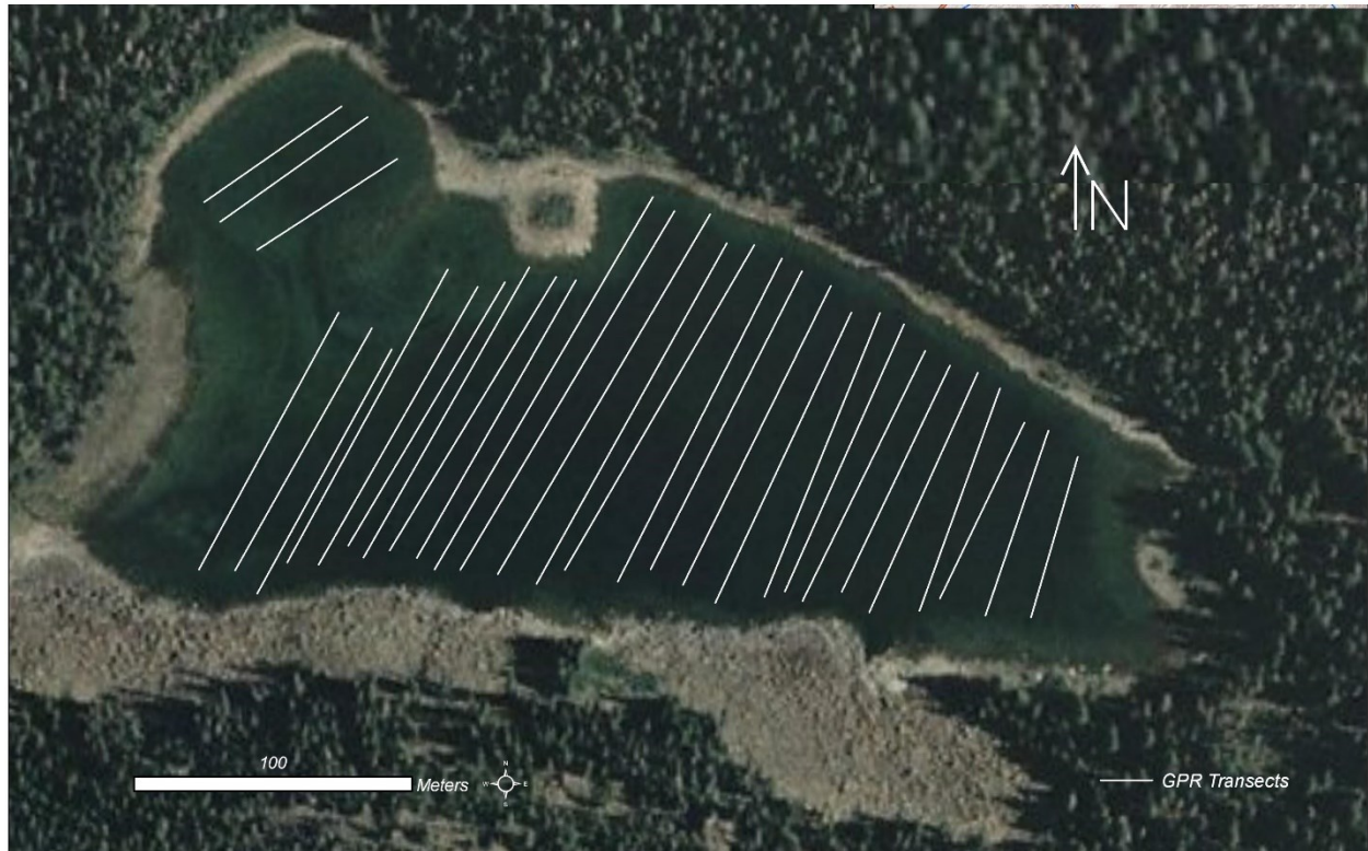
Figure 5: Placement of the GPR transects after correction for locations, where GPS points were located at the beginning and end of each transect.
