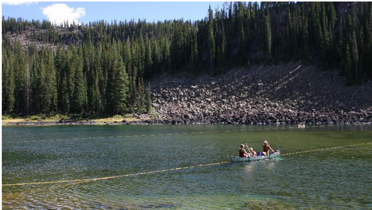
Figure 2: Collecting GPR in a canoe, following a water-ski rope, which floats on the surface.
