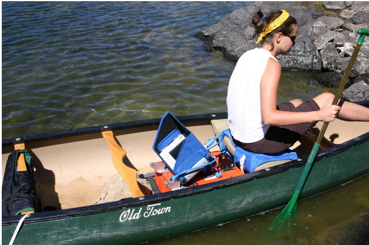
Figure 3: The 270 MHz antenna on the canoe bottom, with the control system resting on it.
