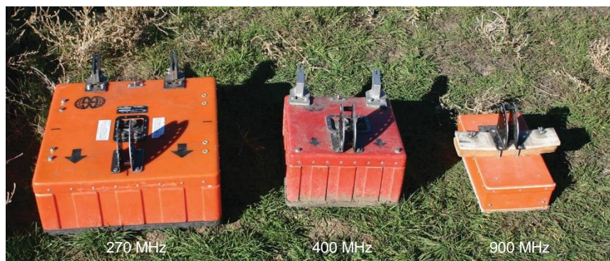
Figure 2.2 Some GPR antennae commonly used in geoarchaeological investigations with the 270 MHz energy traveling deepest in the ground (up to 6 m), with the least feature and
