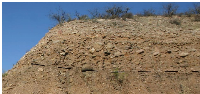
Figure 2.5 The interface tested with two different reflection profiles using different frequency antennae. The stratigraphic interface is at the boundary between an upper cobble and
