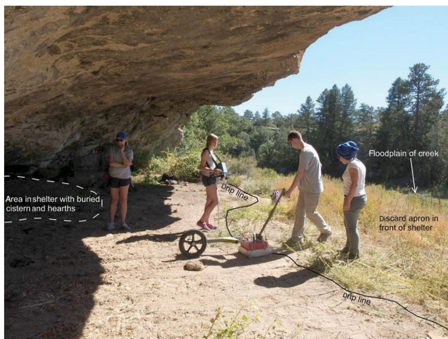
Figure 8.1 Collecting 400 MHz reflection profiles in the Cherry Creek Canyon Rock Shelter of Colorado.
