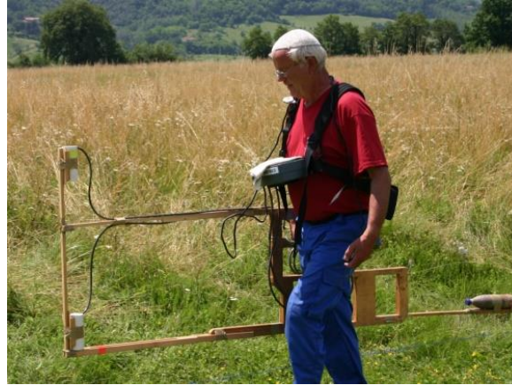
Figure 3.7: Cesium gradiometer with two sensors, supported by a homemade carrying device constructed by Helmut Becker for ease of packing and traveling.
