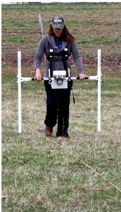
Figure 3.2: A Bartington dual sensor magnetic gradiometer system.
