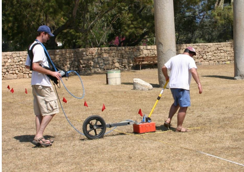
Figure 2.2: A GSSI SIR-3000 GPR system with a 400 MHz antenna and survey wheel.
