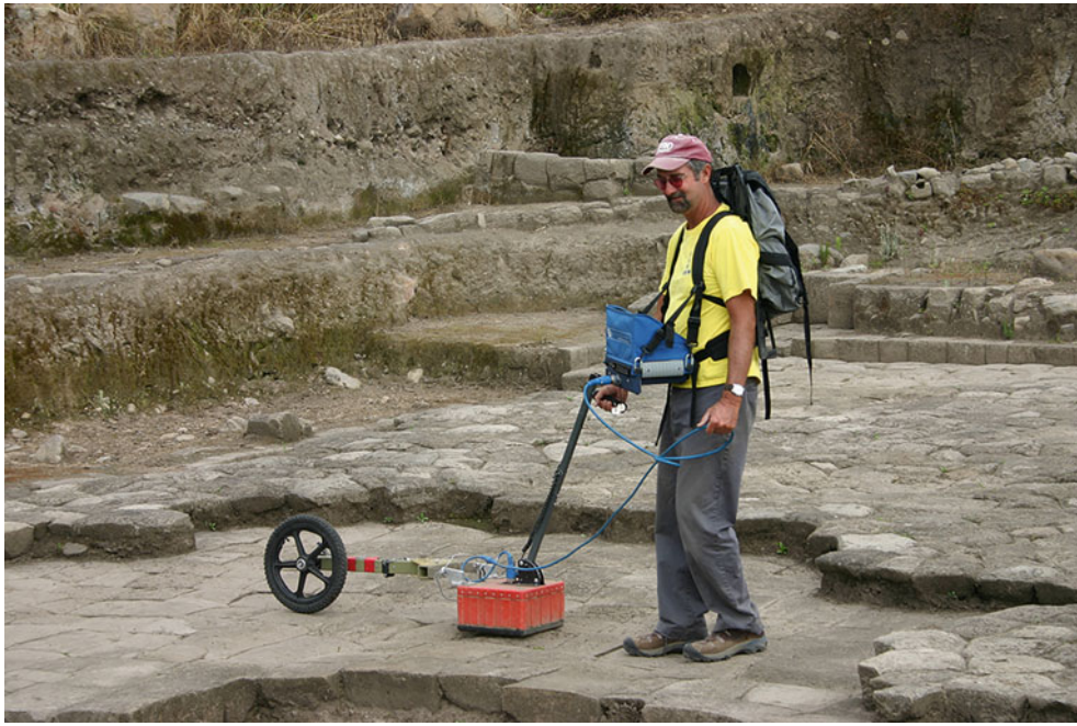
Ground-Penetrating Radar, Fig. 1 GPR equipment including 400 MHz transmission and reception antennas in the fiberglass box, attached survey wheel for distance measurement, and the radar control
