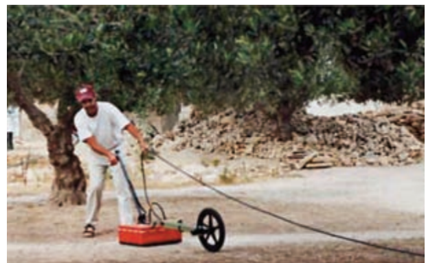
Figure 10-5: Collecting reflection profiles in an olive grove in Tunisia. The 270 MHz reflection profiles were used to test what was under the surface in an area where water did not pool on the ground during rainstorms, suggesting a void space below.
