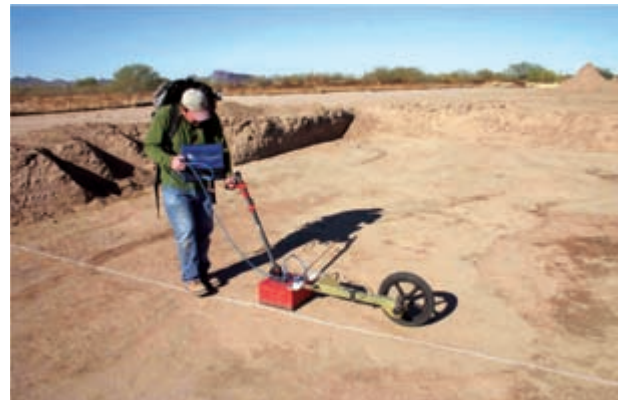
Figure 9-23: Collecting reflection profiles at the Rillito Fan site in Tucson, Arizona, with 400 MHz antennas. About a meter of overburden sediment had to be removed, as the sediment at this location is electrically conductive and attenuates radar energy within about a meter of the ground surface.
