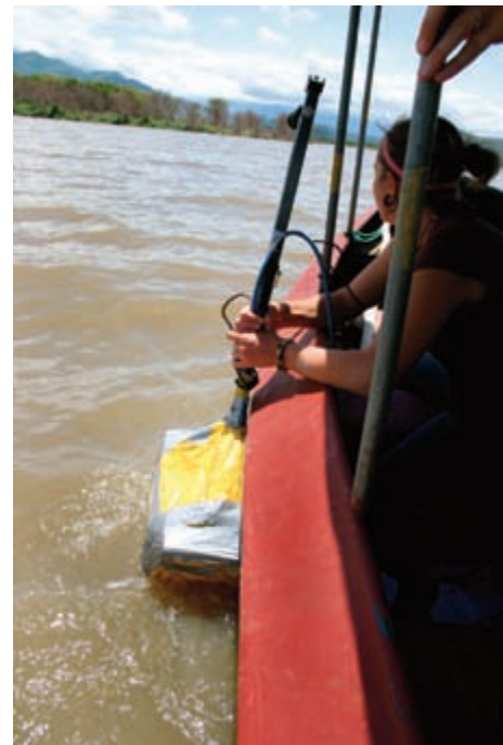
Figure 12-16: Attempting to collect reflection data holding 400 MHz antennas wrapped in plastic, along the side of a metal boat in Lake Chamo, Ethiopia. No reflections were recorded except for those from the metal boat side.
