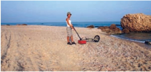
Figure 4-13: Collecting GPR data on the beach at Ashkelon, Israel. Here 400 MHz antennas were used to map large bedrock slump blocks, some of which can be seen on the surface, having fallen from the sea cliff that is located just outside the frame (to the left) of this picture.
