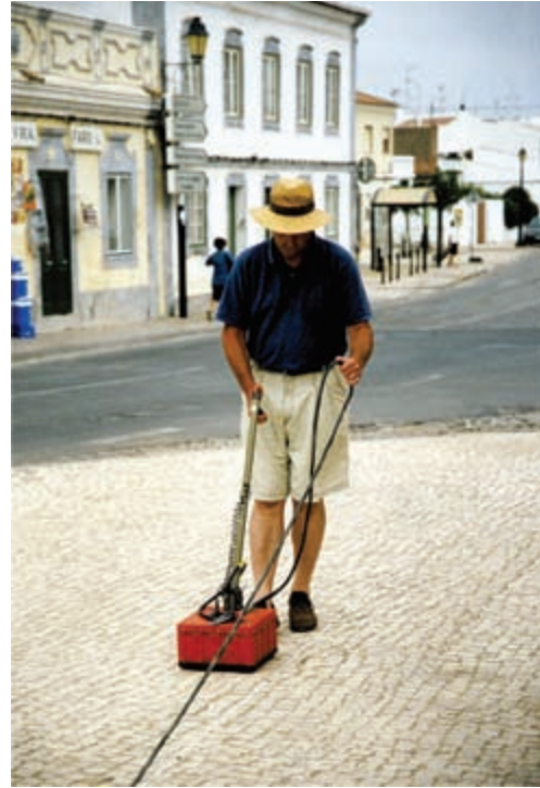
Figure 5-11: Collecting a GPR profile on limestone cobbles and an asphalt surfaced road. This profile was started on limestone cobbles, where the antenna is located in this photo, and then moved onto the asphalt-surfaced road in the background using 400 MHz antennas, in Castro Marim, Portugal. The profile collected here is shown in Figure 5-12, with the curb that produced the air waves in Figure 5-8 in the background.
