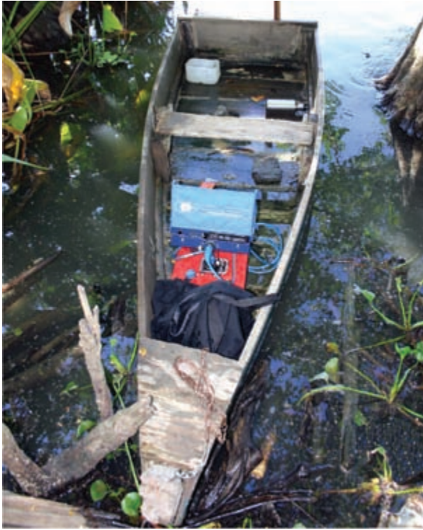
Figure 12-14: GPR equipment placed in a very leaky homemade boat. This very scary project was in Lake Saladilla, Dominican Republic.
