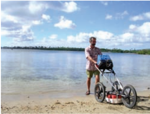
Figure 6-16: Testing saltwater attenuation on a beach. This test was done on a coral beach at Pearl Harbor, Hawaii. The antennas were placed in the saltwater and then moved up the beach to determine the distance from the saltwater-beach interface where there remained radar energy attenuation.
