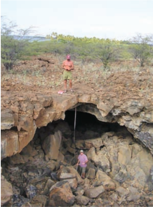
Figure 10-11: Measuring the ceiling thickness and void space in a very large lava tube in Hawaii. This lava tube near Kona, Hawaii, contains rubble on the floor from ceiling collapse, which allowed us access to this long, sinuous tunnel.
