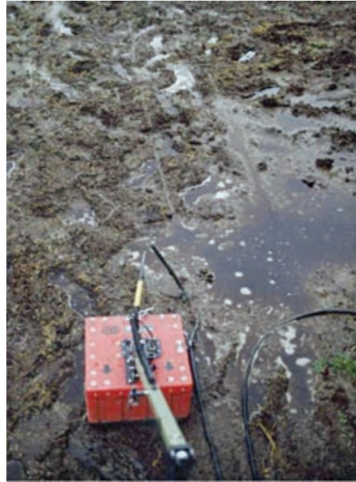
Figure 6-9: Attempting to collect GPR data in saturated cow manure, using 400 MHz antennas near Salinas, California. There was absolutely no energy penetration whatever in this ground, due to the very high conductivity of the medium.
