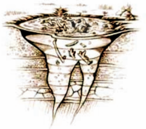
Figure 4-17: Schematic image of an oil seep. Seeps of this conical shape are common at the La Brea Tar Pits in Los Angeles, California, where oil seeps upward along fractures from depth; the cone shape is wider at the top due to bank slumping and struggling animals mired in the oil.
