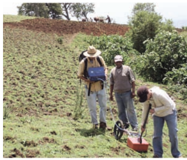
Figure 5-9: Recently plowed fields in highland Ethiopia. This recent disturbance produced a very difficult surface on which to collect GPR data, as the antennas were always changing their coupling characteristics.
