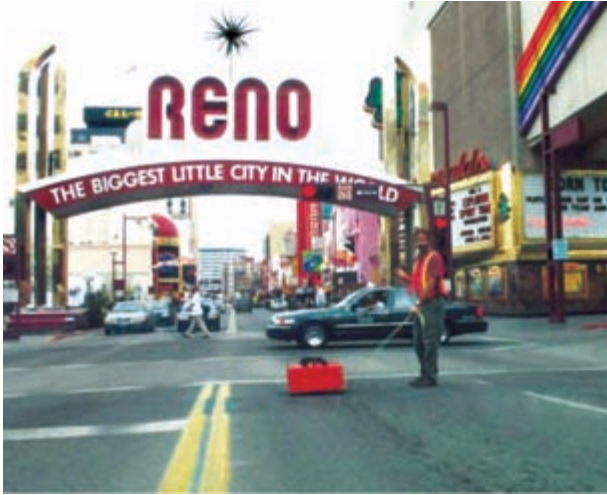
Figure 5-3: GPR profile collection over a concrete road surface in Reno, Nevada. The road surface had metal reinforcing mesh embedded in it, which interfered with energy penetration. Data collected with 200 MHz antennas.
