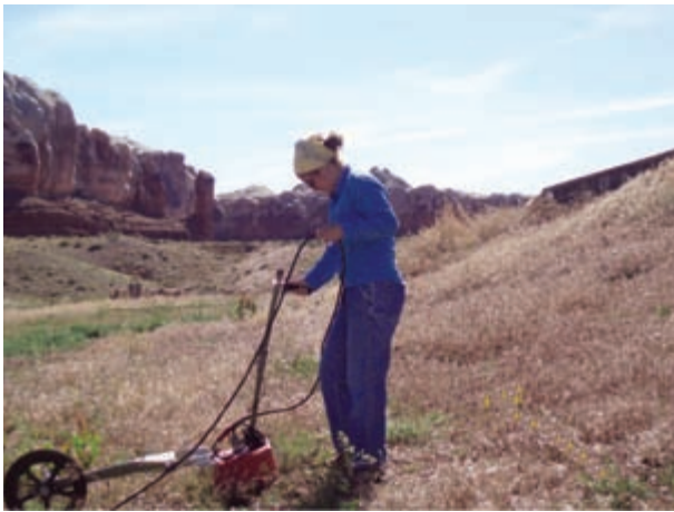
Figure 9-11: Collecting reflection profiles along the north side of a greathouse. This is the Bluff Greathouse (just visible on the right side of the picture) where 400 MHz antennas were used to collect data in order to map an adjacent earthen terrace feature. Image courtesy of Sarah Lowry.
