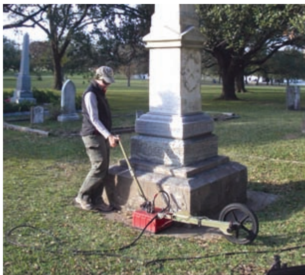
Figure 8-1: Collecting 400 MHz reflection data at San Jacinto cemetery, Texas. Antennas had to avoid the monuments, which complicated profile collection. Image courtesy of Jennie Sturm.
