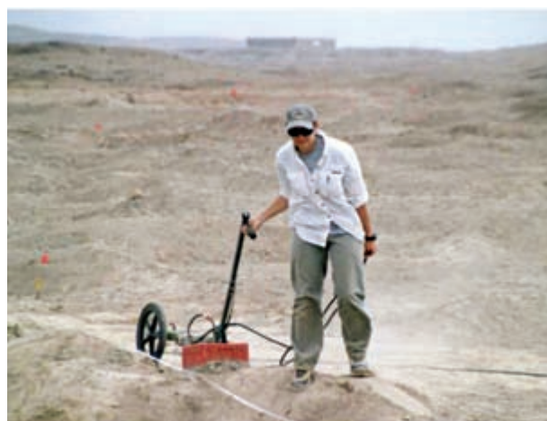
Figure 6-5: Collecting GPR data in very dry sand. On the north coast of Peru it has not rained in decades, and the sand is very dry.
