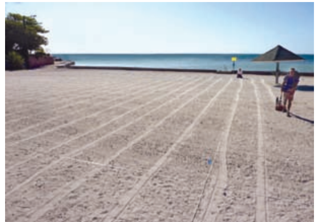
Figure 4-7: Collecting GPR data along the beach at Key West, Florida. Here the 400 MHz antennas were used to discover what is below this imported beach sand, which covers a complex buried topography incised into bedrock.
