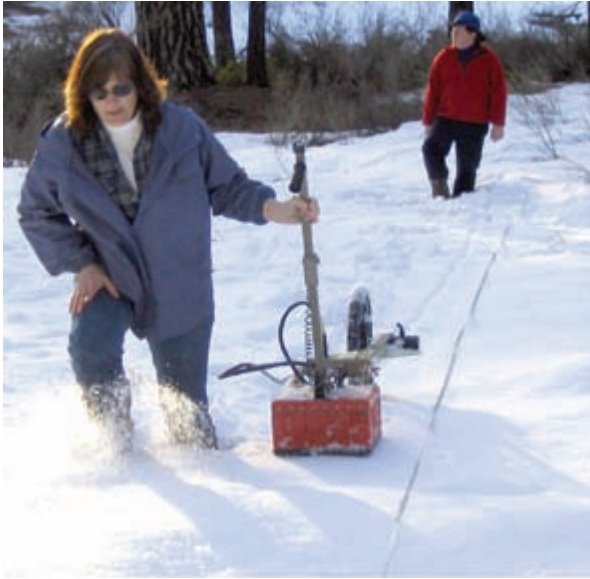
Figure 12-4: Collecting 400 MHz reflection profiles in deep snow in central Oregon. The survey wheel slipped, and many air waves were recorded as energy moved within the snow layer and reflected off air pockets within the snow.
