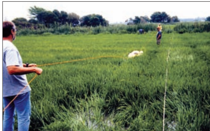
Figure 12-6: Reflection profile collected in an inflatable canoe across a flooded rice paddy in coastal Portugal. All energy was attenuated in the somewhat brackish water of the paddy, but good reflections were generated as soon as the antennas moved on shore. Data collected with 400 MHz antennas
