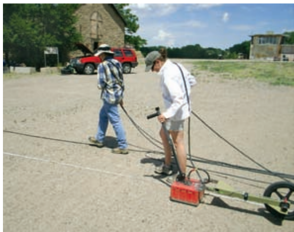
Figure 5-14: Collecting GPR data at the Goodnight Barn site. The 400 MHz antennas were used to collect data around a flat surface created by leveling during gravel-extraction operations near the site in Pueblo, Colorado.
