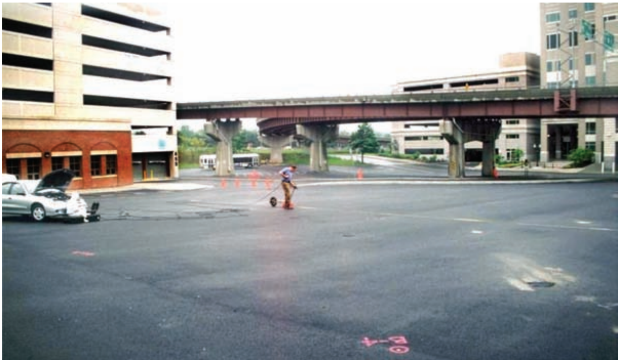
Figure 7-14: Collecting GPR profiles in a parking lot in Albany, New York. A number of interesting historic buildings were discovered.
