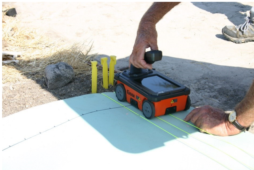
Figure 2: Collecting profiles with the 2.6 GHz antenna on a yoga mat, with strings along which the antenna was moved spaced 5 cm apart. A laser in the antenna allowed it to be moved along the strings in a perfectly straight line, with black grid edges showing the start and end of each profile. In this fashion all grids were exactly 150 cm wide and all profiles perfectly straight and separated from each other by 5 cm.
